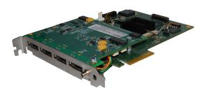
The iSAFT Quad SpaceFibre Interface Card is an advanced PCIe interface, supporting SpaceFibre simulation with built-in recording function. It is suitable for multiple applications in the space sector, including Data Front-Ends, EGSE/SCOEs.
