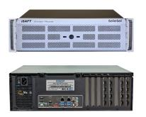
The iSAFT SpaceWire Front-End is a SpaceWire data interface with advanced asynchronous transmission and traffic generation capabilities that simulates SpaceWire devices or Instruments, enabling S/C integration tests before the availability of Flight Models.
